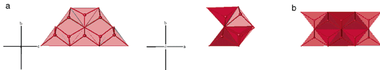
Figure 5. (a) OA 4 tetrahedra edge-sharing pattern in Bi 4.6 Ca 1.1 VO 10.5 viewed perpendicular to the a axis and the c axis. (b) OBi 4 tetrahedra edge-sharing pattern in \delta -Bi 2 O 3 viewed perpendicular to the cubic face diagonal.
